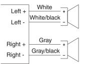
Left and right wiring diagram
